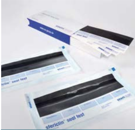
Seal test in application
