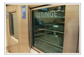
We recommend monitoring every shelf on every washer each day for a machine release and using a minimum of one Wash-Checks per load for routine monitoring throughout the day.
