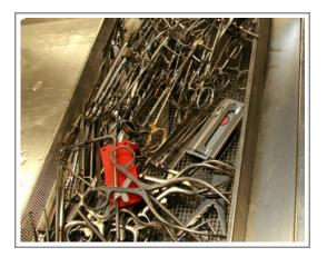
Place basket on a shelf in the washer. Vary positions and shelves of Wash-Checks placement cycle to cycle.
